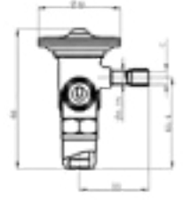
Valve Body - Connection Type: flare/solder/solder
